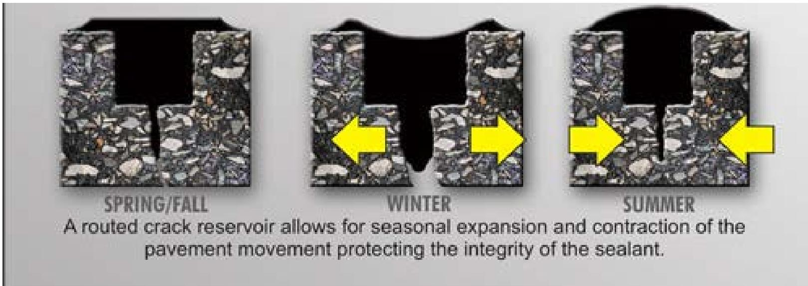
**AS THE CRACK MOVES, THE MATERIAL BONDS TO THE EDGES AND MOVES AS WELL**
